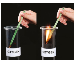
Oxygen relights a glowing splint
