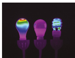
The heat given off by an old-fashioned (incandescent) bulb, a light emitting diode (LED) and a compact fluorescent bulb
